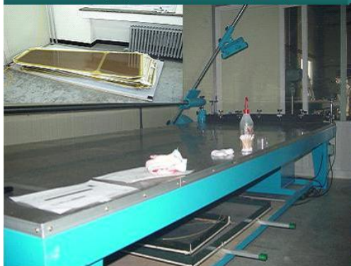
Silk screen method for graphite coating (100 ~ 200 k \Omega /square)
